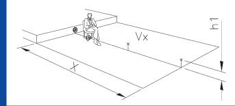
V<sub>x</sub>= Velocity at a distance of 0.7 m from the diffuser  $h_1$ = Distance of 0.1 m above the ground  $\Delta t$ = -6 °C
